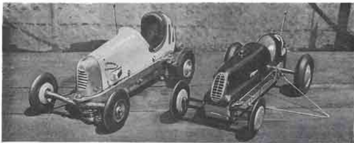
Facer at left rides a flanged steel rail around the miniature track. Steel wire on model at right fastens to a cable for faster cable-track racing. World's record cable car zoomed the course at more than 114 miles an hour.
