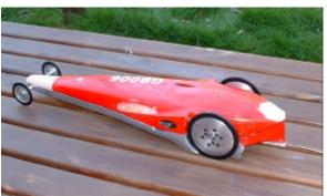
View of the car after repairs to the tail and modifications to the nose to accommodate the lengthened wheelbase, prior to refinishing. Balsa top covered with glass cloth and epoxy resin allows easy modification.
