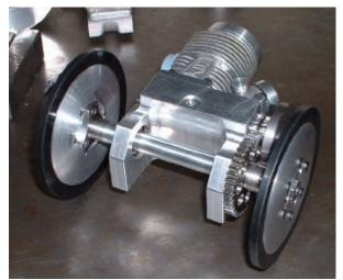
Lightened engine mount, 2.5cc wheels and lightened driven gear apparent in this view
