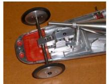
View of the front suspension with adjustable damping.
