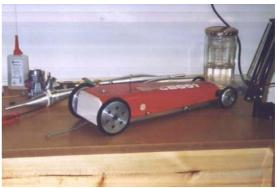
The car after surgery to the back end and prior to re-finishing with glass & epoxy.
