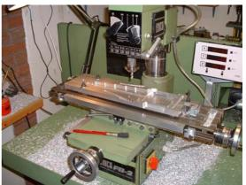
The lower pan, part way through the machining operation. 3 axis digital readout proved invaluable during this and other operations. An invaluable piece of equipment!
