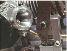
A nicely machined venturi using a needle valve assembly from a 3,5cc CMB marine engine. Detail from an early car by Mart Sepp.
